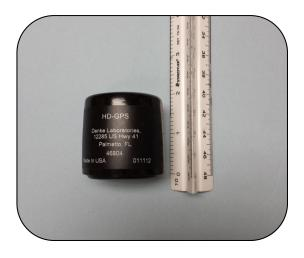
The HD-GPS-TIMING antenna covers the GPS L1, GLONASS L1 and SBAS (WAAS, EGNOS, & MSAS) bands from 1575-1606 MHz. It can be ordered in an NMO mount or with a threaded section for pass thru mounting with a pigtail.
